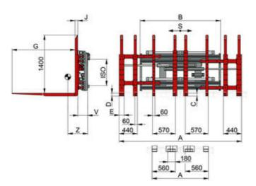
with independent sideshift - for 2 or 4 pallets side by side or 4 or 8 pallets - 2 hydraulic functions
